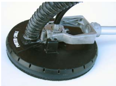
FIGURE 3. Articulating sanding head of the SVRS with extractor shroud
